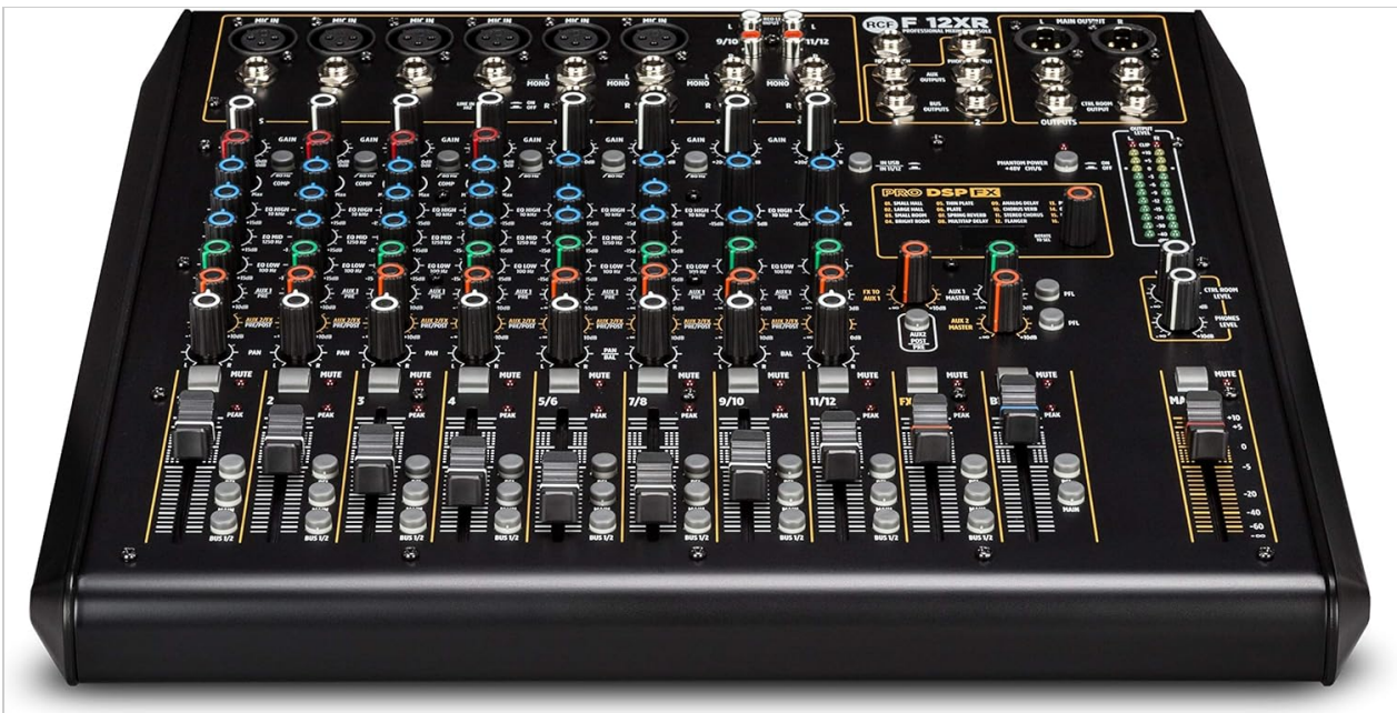
Figure 4.1: Top-down view of the RCF F12 XR control surface. This image clearly displays the layout of all controls, including individual channel strips, the master section, and the DSP effects module.
