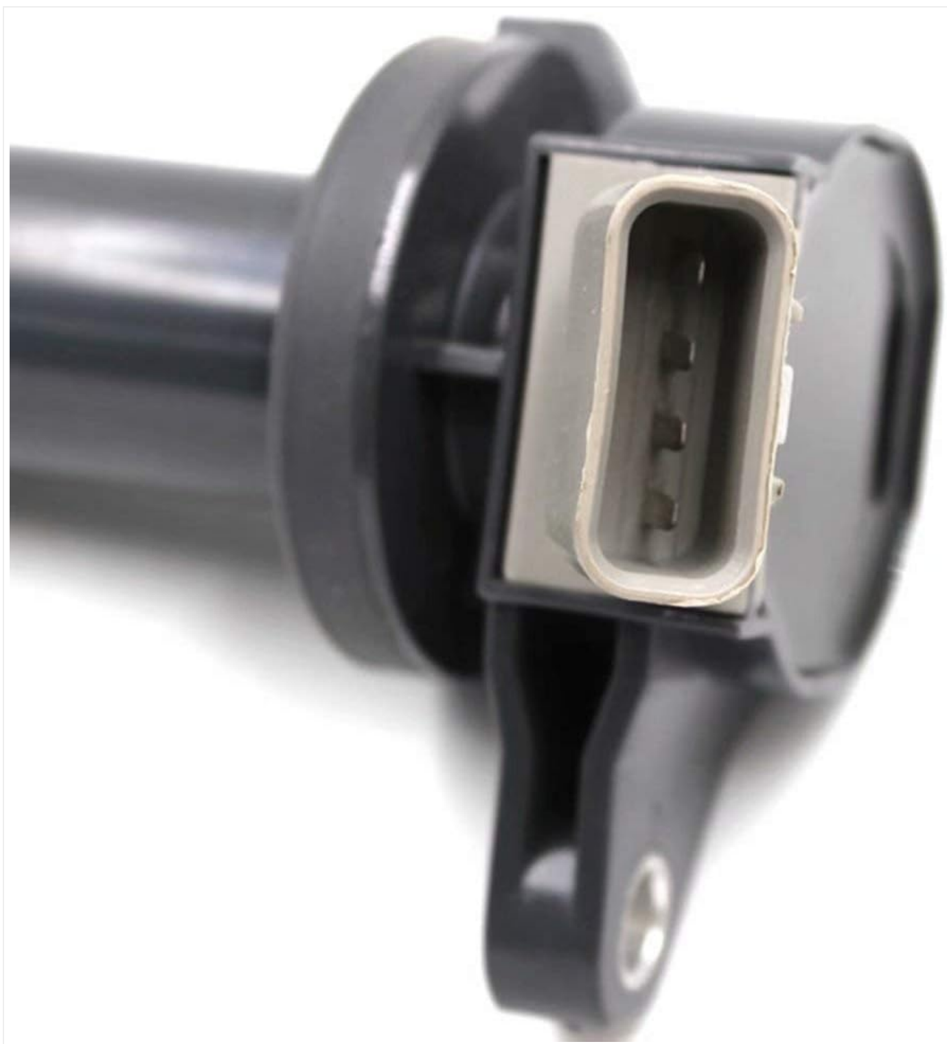
Figure 4: Close-up view of the electrical connector pins on the ignition coil. This detail is important for ensuring proper alignment and connection with the vehicle's wiring harness.
