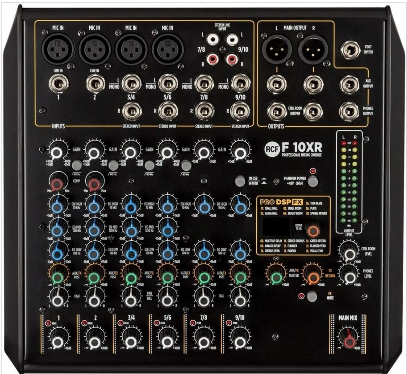
Figure 1: Overview of the RCF F-10XR mixer's top panel, highlighting the various input and output connections, along with the main control sections for each channel, effects, and master outputs. The image clearly shows the MIC IN, LINE IN, STEREO LINE INPUTs, MAIN OUTPUT, CTRL ROOM OUTPUT, PHONES OUTPUT, and AUX OUTPUT sections, as well as the individual channel strips with GAIN, EQ, AUX/FX, PAN/BAL, and LEVEL controls. The PRO DSP FX section and the main mix fader are also visible.
