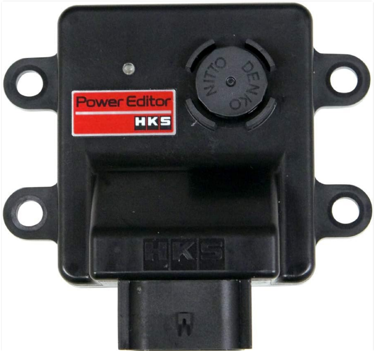
Figure 3.2: Close-up view of the HKS Power Editor main unit, showing its compact design and connection ports.
