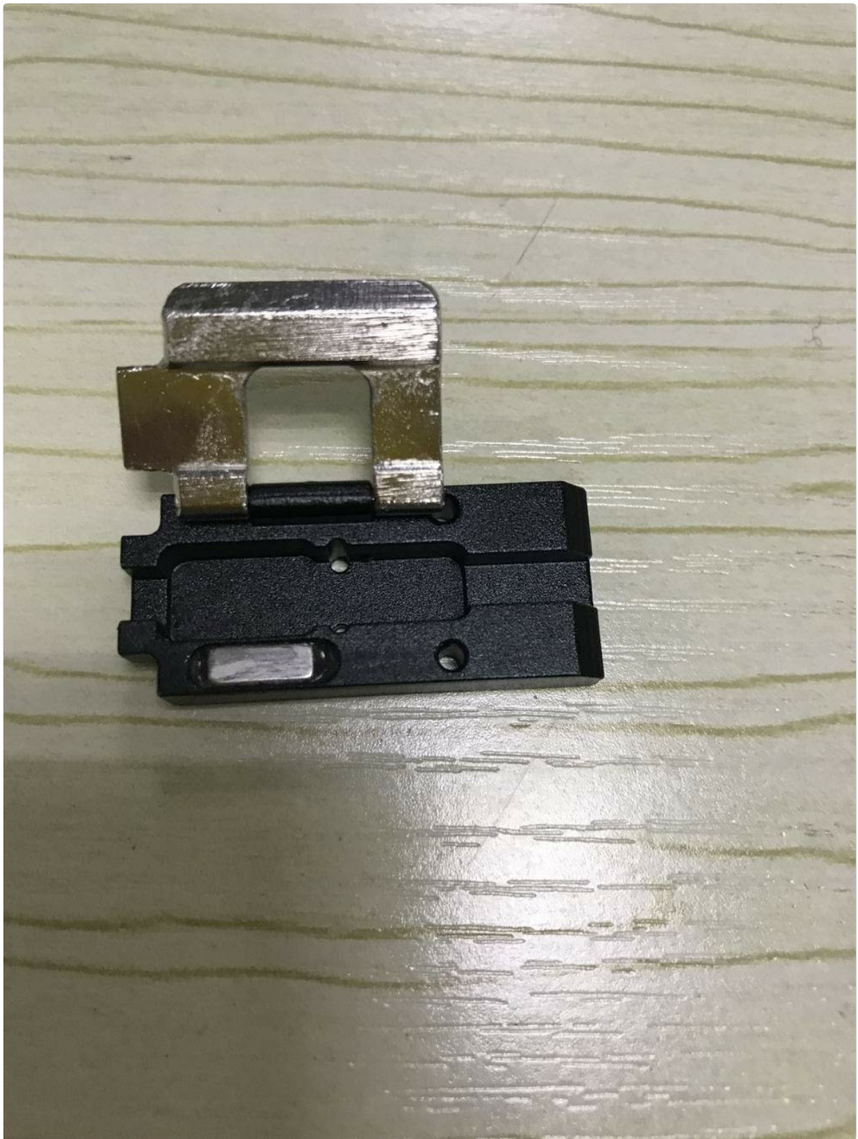
Figure 2: Side view illustrating the design of the fiber holder, showing the clamping mechanism for securing the fiber or connector.
