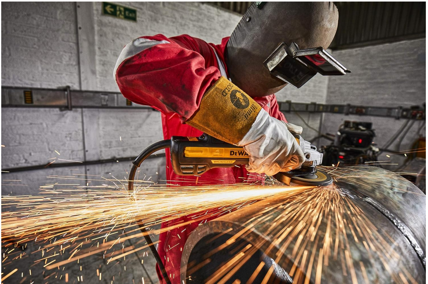
Figure 3: DEWALT DWE4002-B5 Angle Grinder in operation. This image illustrates the grinder being used on a metal pipe, producing sparks, highlighting the need for proper PPE and work area safety.
