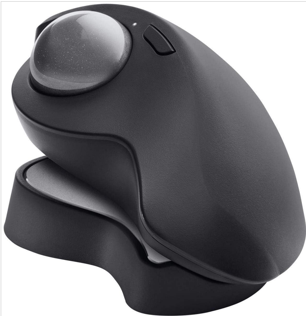
Figure 4: Side view illustrating the adjustable hinge mechanism of the MX Ergo Plus for ergonomic customization.
