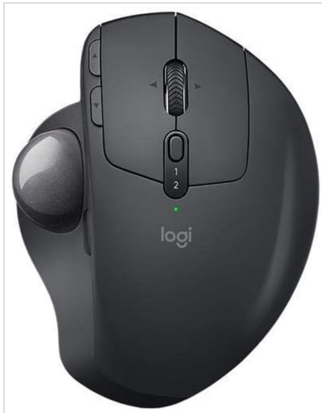
Figure 5: Top view of the MX Ergo Plus, detailing the placement of the scroll wheel, Easy-Switch buttons, and forward/backward buttons.
