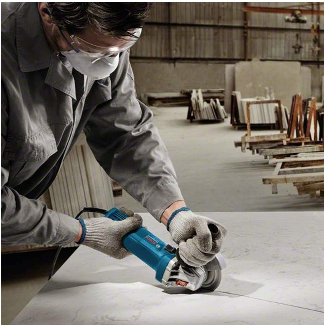
Image: A user demonstrating the use of the angle grinder for cutting or grinding on a flat surface, emphasizing proper grip and safety gear.
