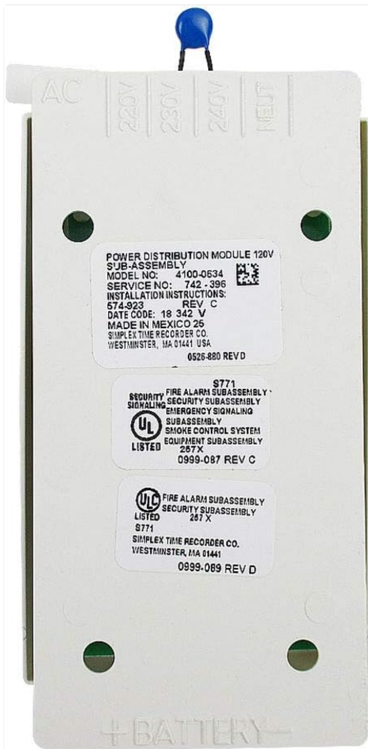
Figure 3: Back view of the Simplex 4100-0634 module, displaying product labels, model number, installation instructions reference, and compliance certifications.
