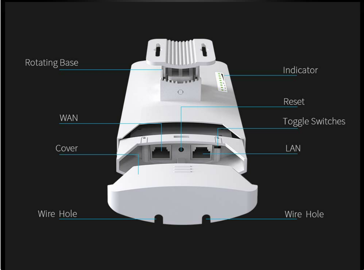
Image: Detailed view of the CF-E113A showing its components: Rotating Base, Indicator LEDs, Reset button, Toggle Switches (STA/AP), WAN port, LAN port, Cover, and Wire Holes.
