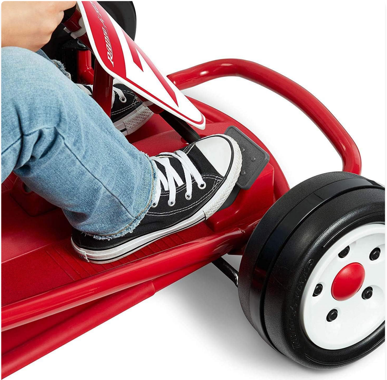
Figure 4.1: The foot pedal controls acceleration.
