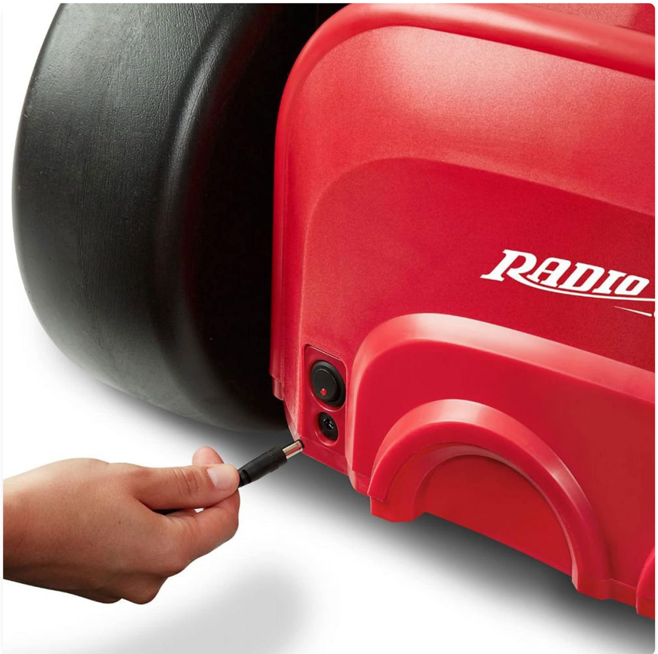
Figure 3.1: Locate the charging port on the rear side of the go-kart for battery charging.
