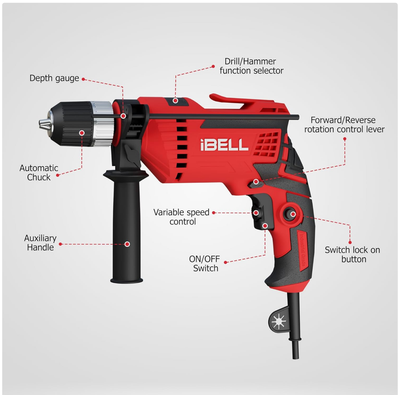
Figure 2: Key components of the IBELL 650W Impact Drill.
