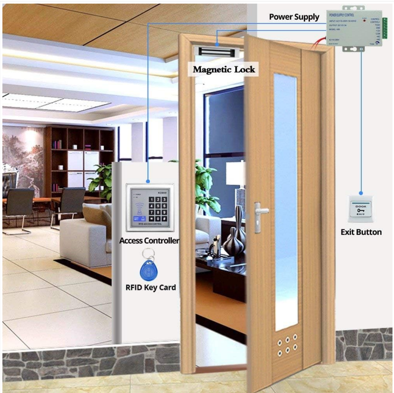
Figure 3.1: System Component Placement. This image illustrates the typical installation of the access controller, magnetic lock, power supply, and exit button on and around a door.
