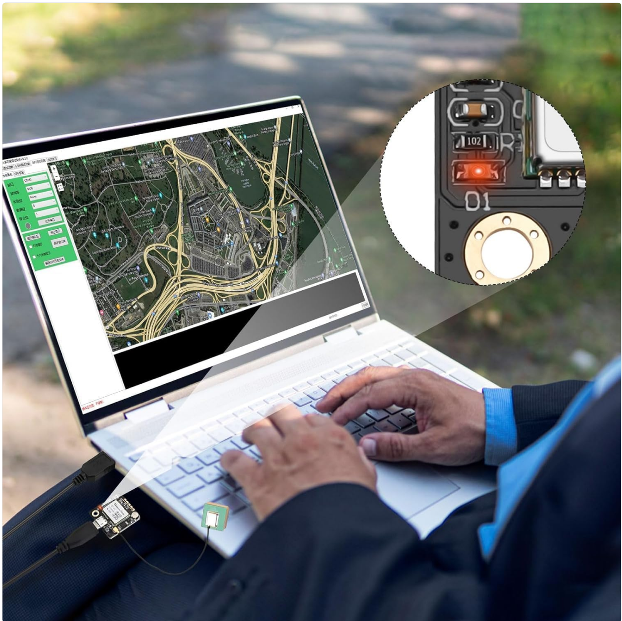
Image 5.1: The GT-U7 GPS module connected to a laptop via USB, demonstrating how positioning data can be viewed on mapping software. The inset shows the module's LED indicator, which flashes upon satellite signal acquisition.
