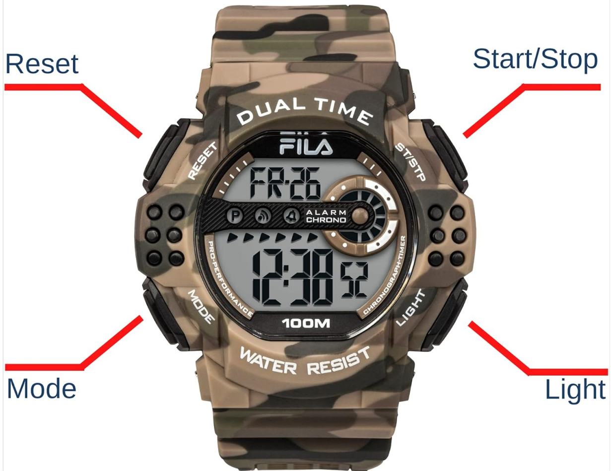
Image 1.2: FILA Digital Watch Model 38-171-003 showing the location of the Reset, Start/Stop, Mode, and Light buttons.
