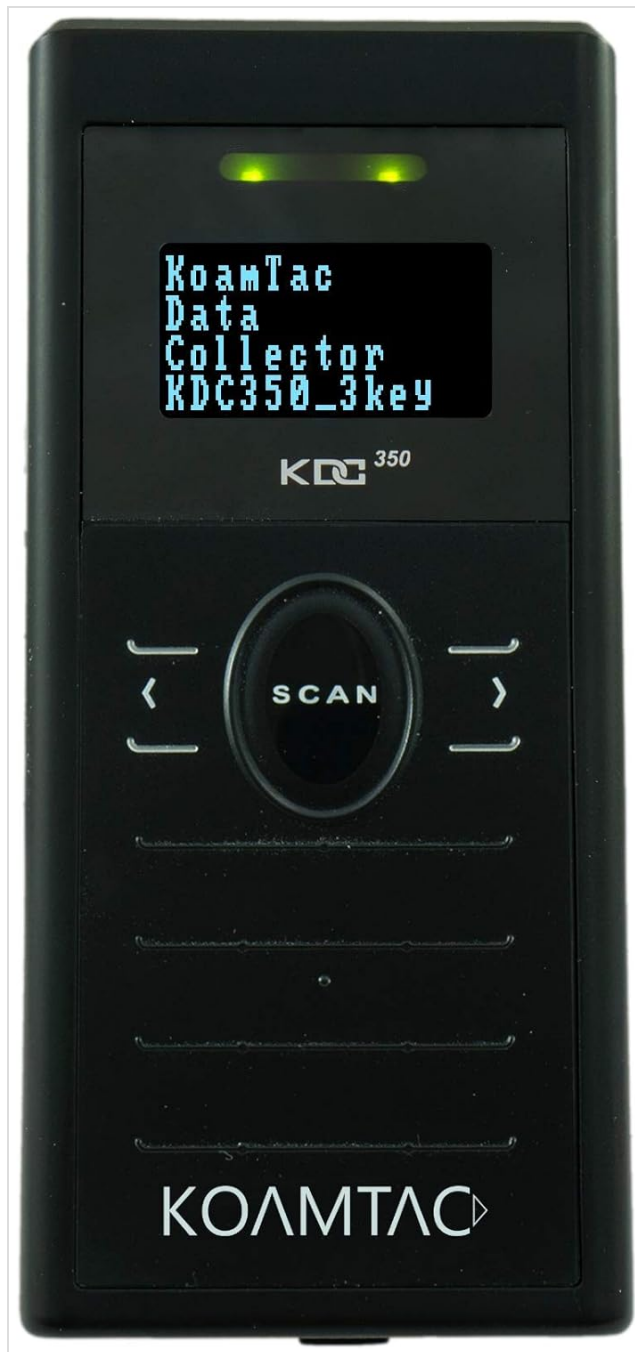
Figure 1: Front view of the KOAMTAC KDC350Ci-G6SR-3K-R2-WFG barcode scanner, showing the display, scan button, and navigation keys.
