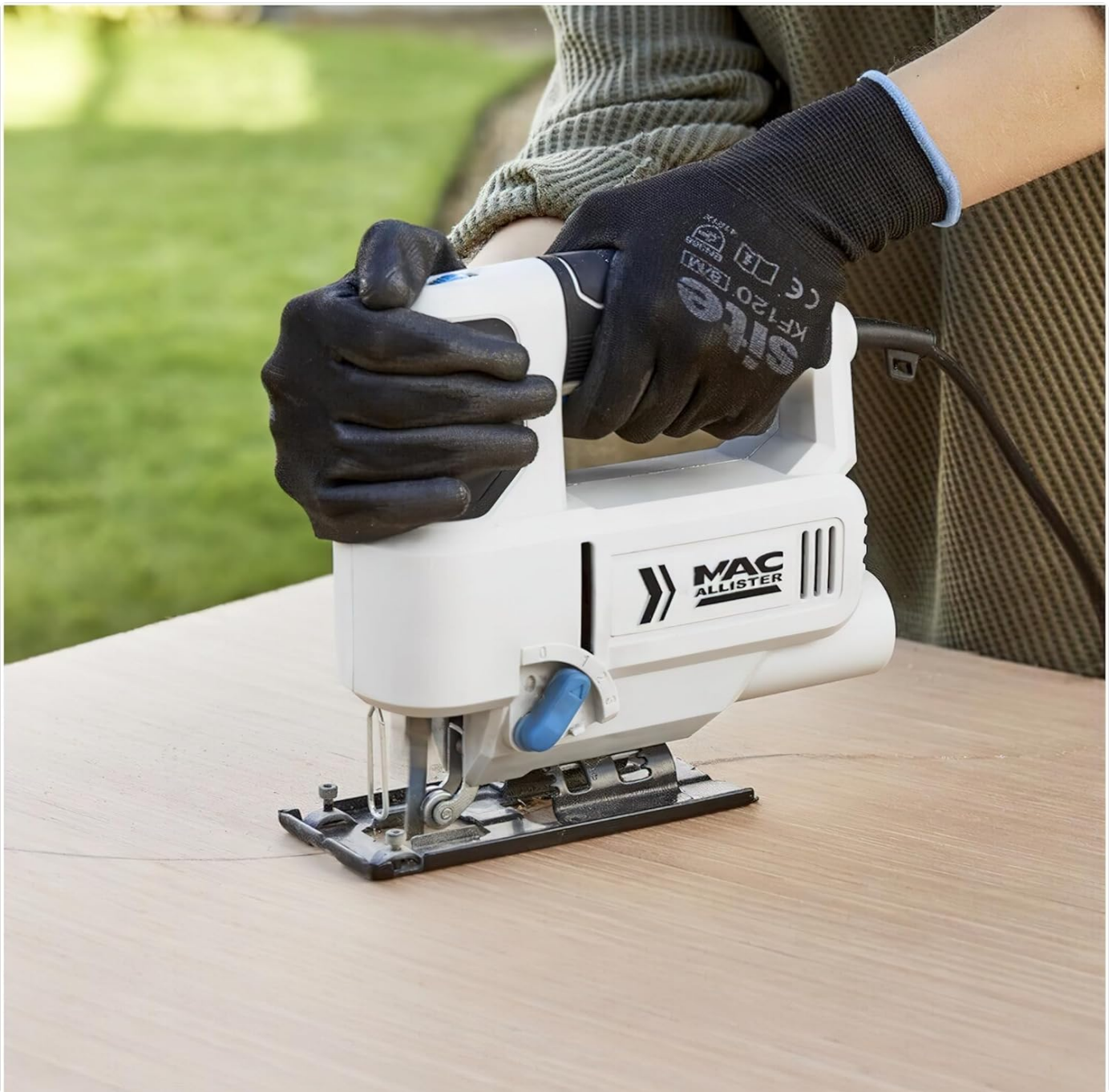
Figure 5.1: A user operating the Mac Allister MSJS600 Jigsaw to cut a piece of wood. This image demonstrates the tool in action, highlighting proper grip and positioning during a cutting task.
