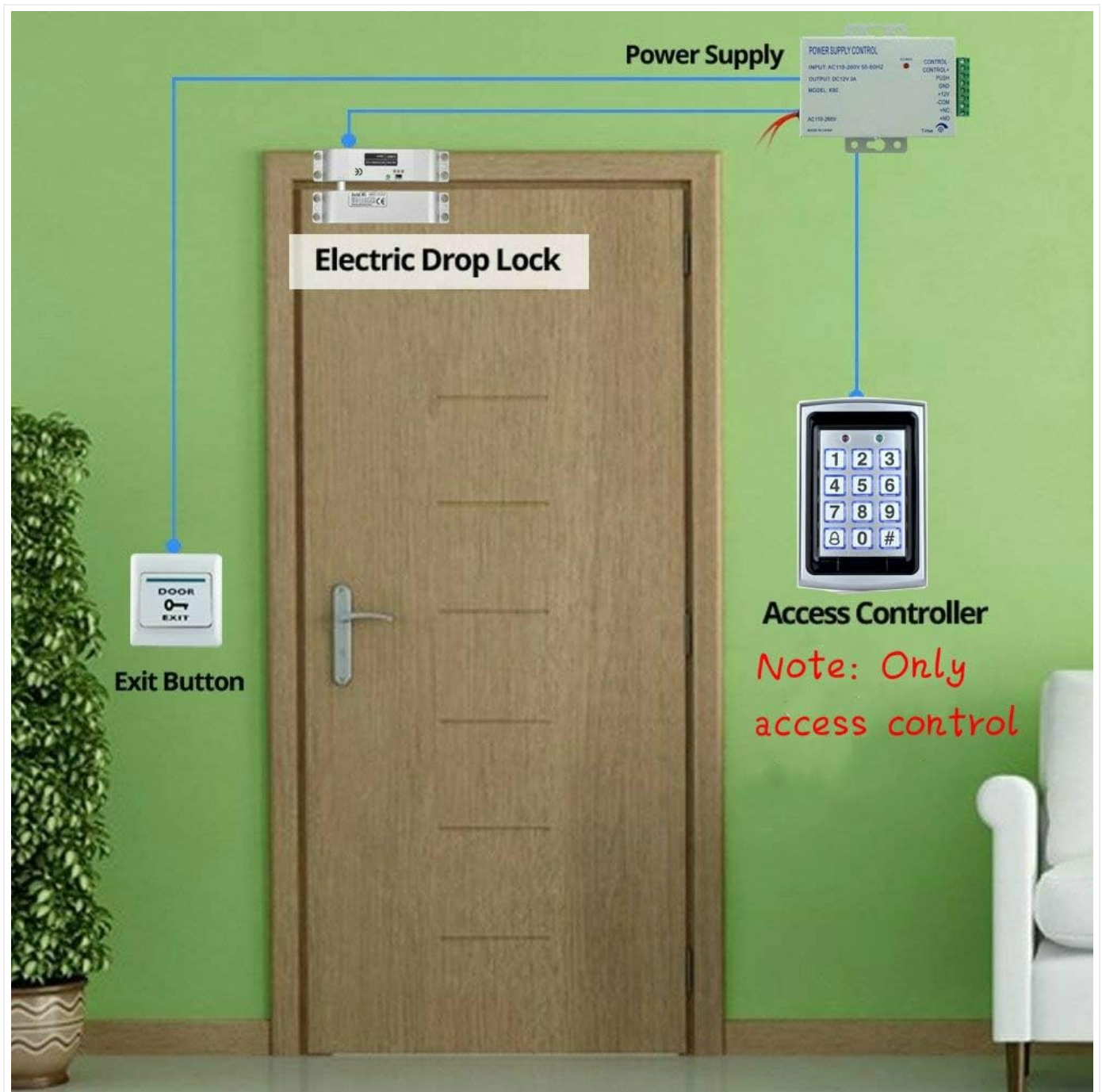
Figure 5: Installation Example. This image shows a typical installation of the access controller next to a door, connected to an electric drop lock and an exit button.
