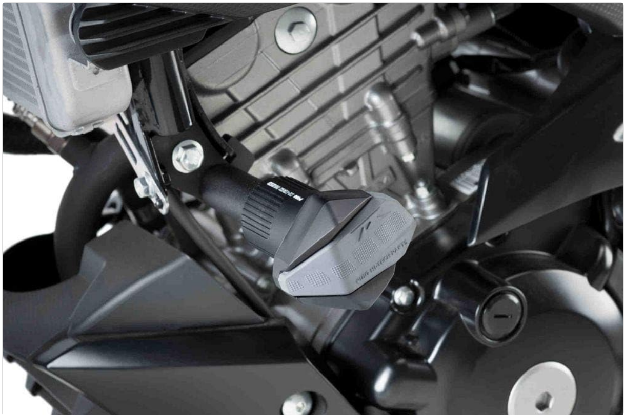
Image 1: Puig R19 Frame Slider securely installed on the side of a motorcycle engine block, demonstrating its position for protection. The slider features a black base with a grey, textured protective cap.
