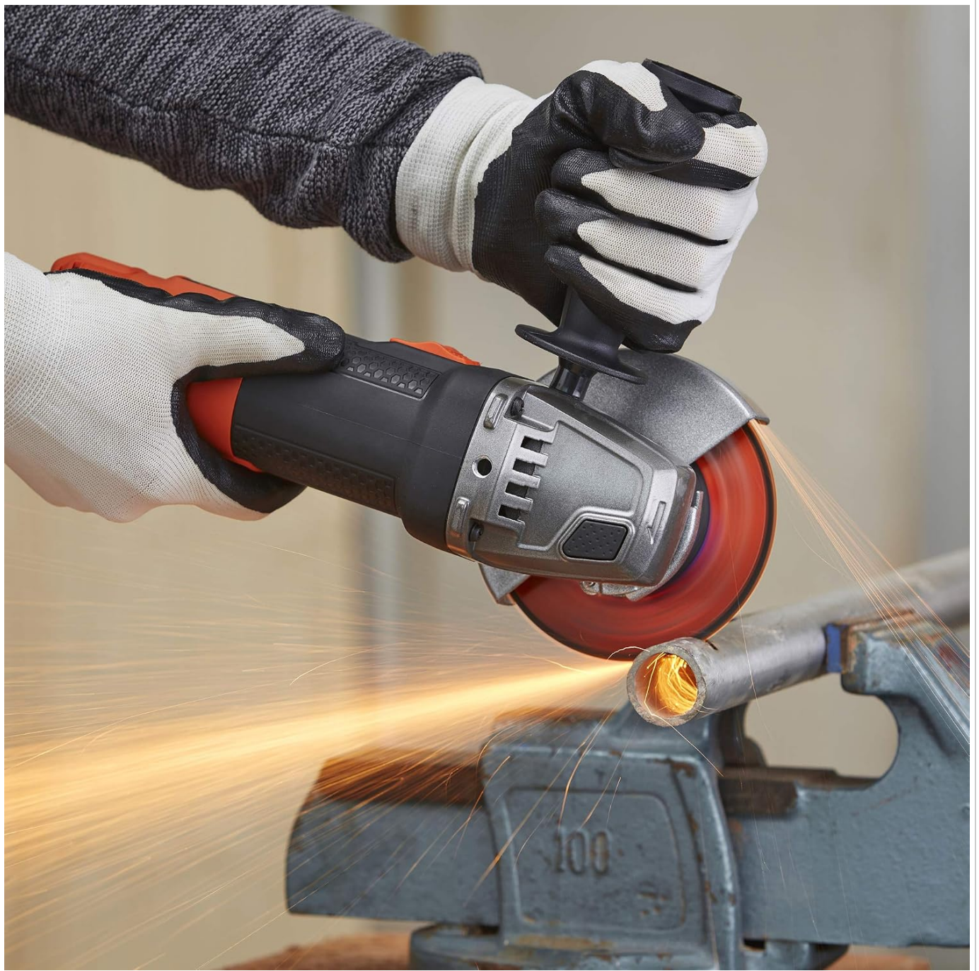
Image: An angle grinder in use, cutting a metal pipe, demonstrating the sparks generated during operation. Always wear appropriate safety gear.
