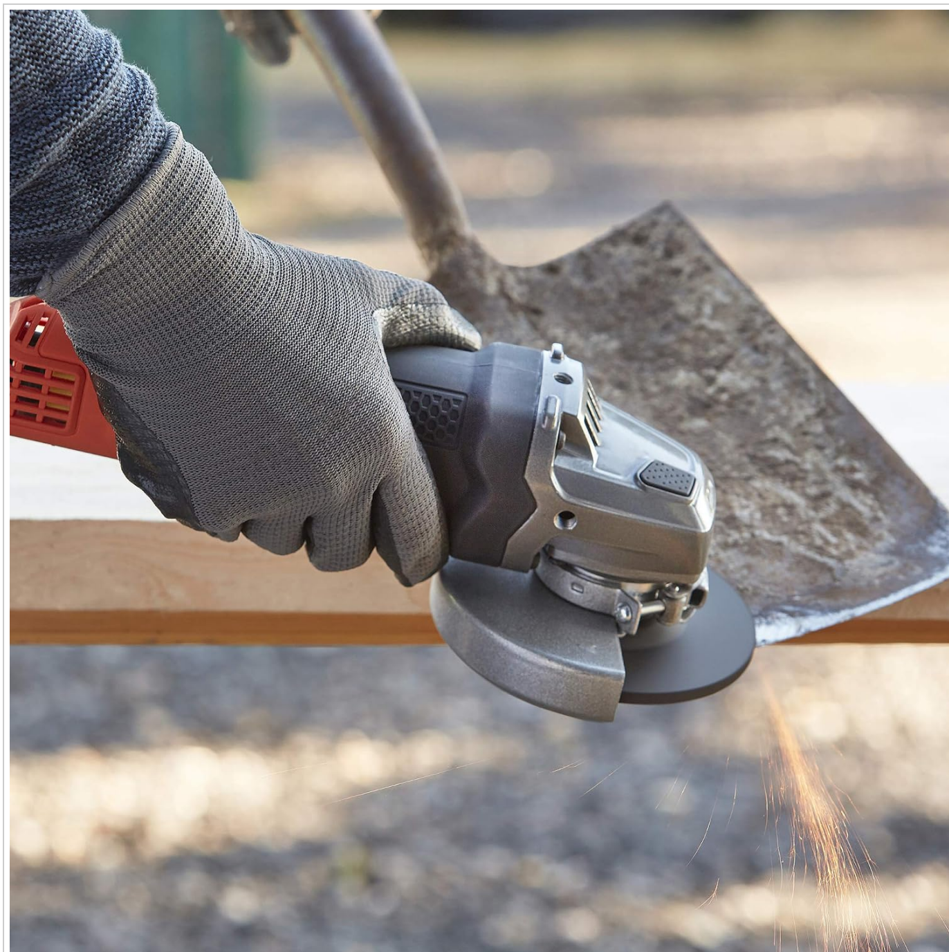
Image: An angle grinder being used to grind a metal surface, possibly a shovel, showing the removal of material. Always secure the item being worked on.
