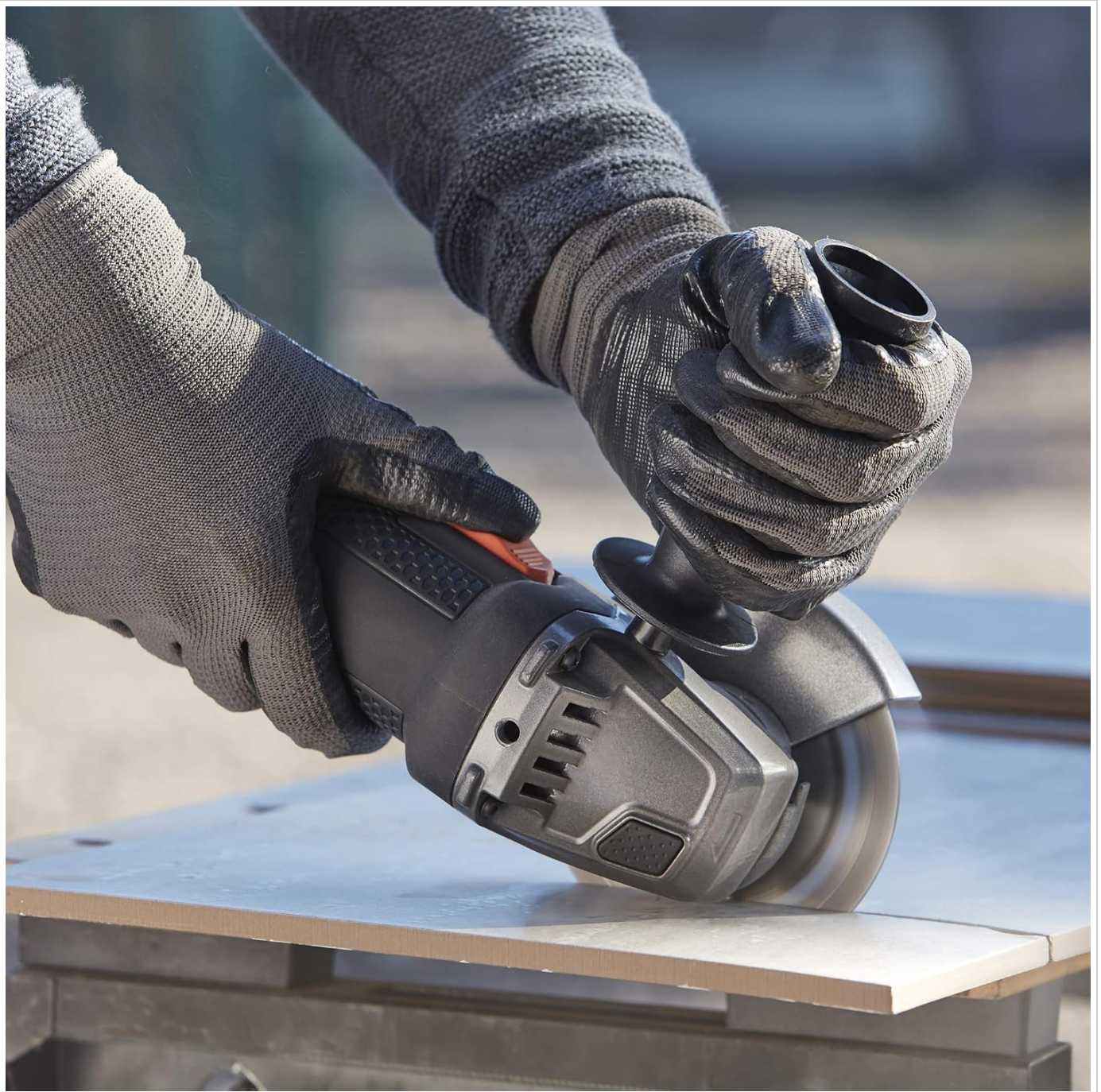
Image: A person using the angle grinder to cut a ceramic tile, demonstrating precision work. Ensure the workpiece is stable.
