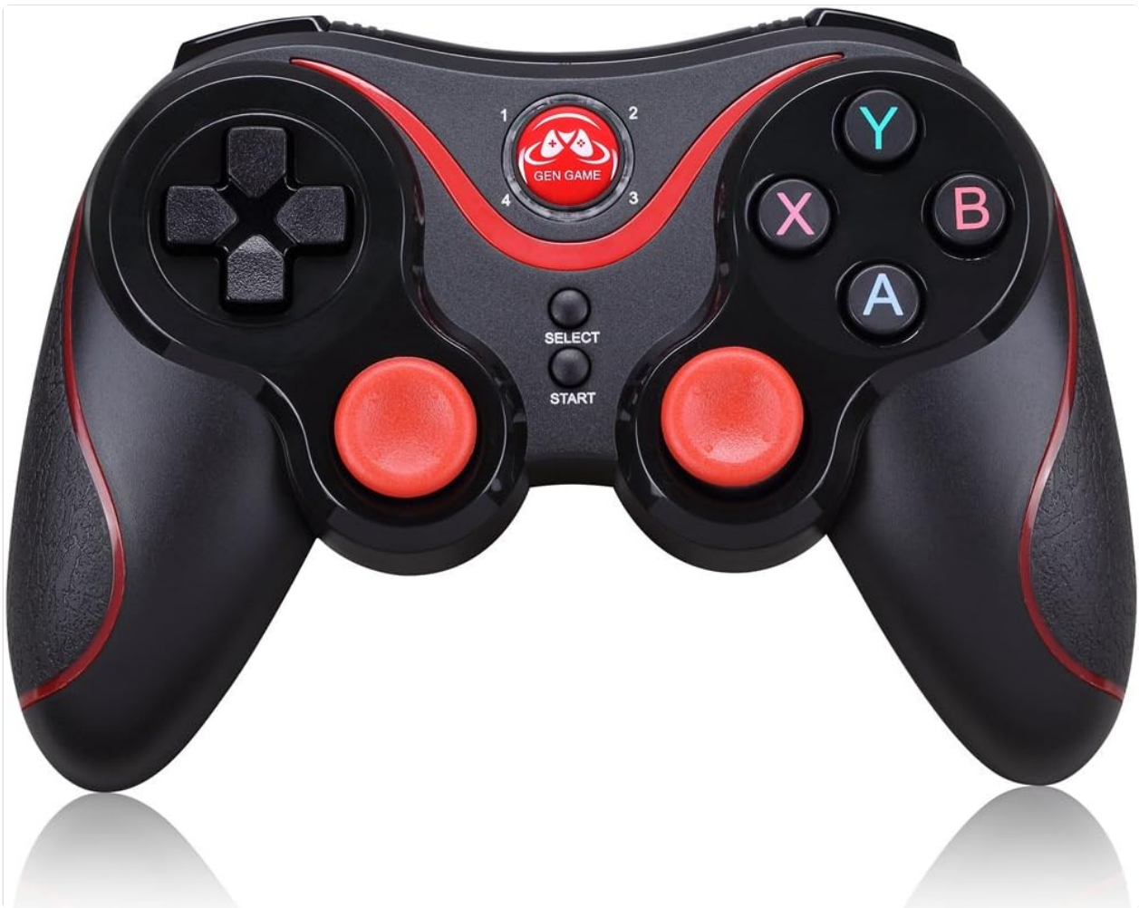
Figure 1: Front view of the Gen Game S5 Wireless Controller, showing the D-pad, left and right analog sticks, action buttons (A, B, X, Y), SELECT and START buttons, and the Gen Game logo.
