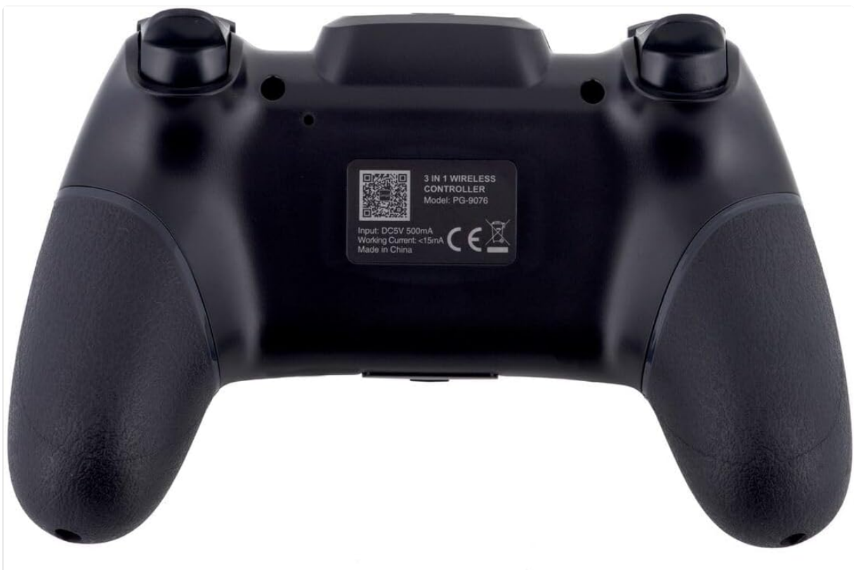
Figure 2.3: Rear view of the controller, displaying the product label with model number, input specifications, and a QR code for additional information or support.
