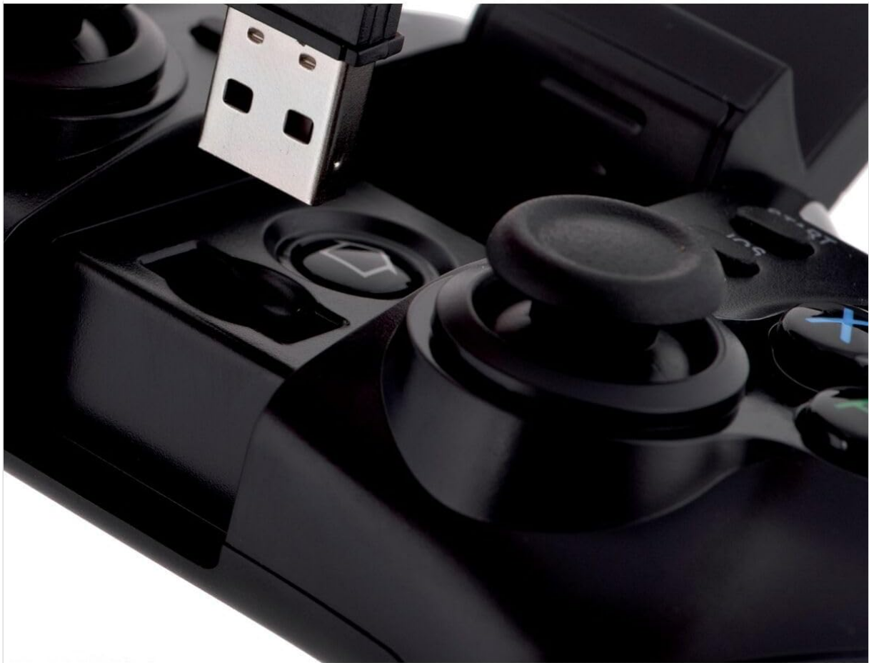
Figure 3.1: The USB dongle (if included with your model) can be inserted into the controller for wireless connection to devices that do not have built-in Bluetooth, such as some PCs or Smart TVs.
