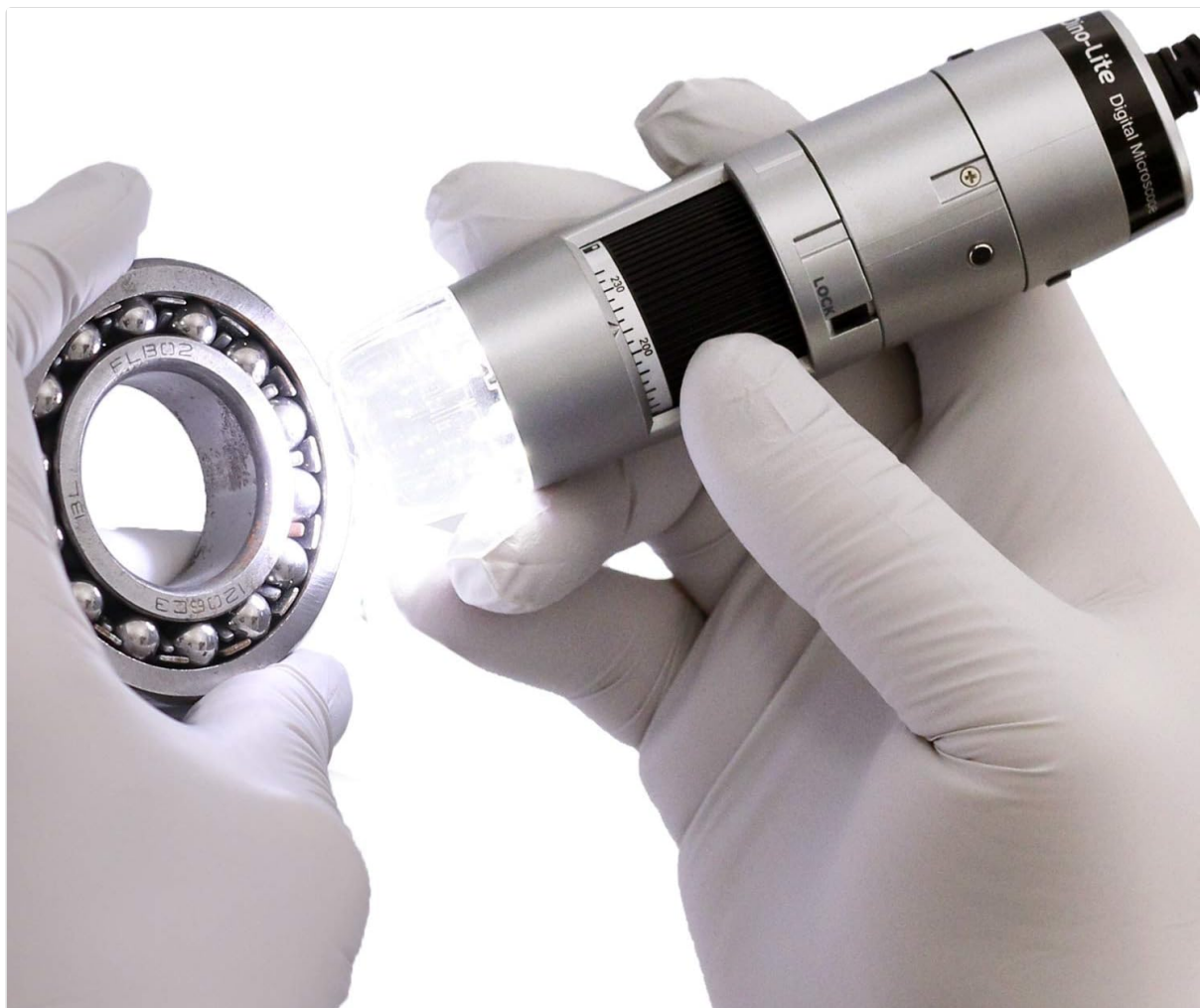
Figure 6: The Dino-Lite microscope in use, demonstrating its ability to inspect small objects with integrated lighting.
