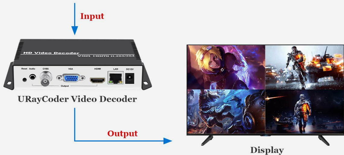
Figure 5: Illustration of multi-channel output, showing four distinct video inputs being decoded and displayed simultaneously on a single screen in a quad layout.
