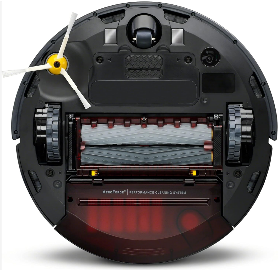
Image: The underside of the Roomba 966, clearly showing the dual multi-surface rubber brushes, side brush, and dustbin compartment, illustrating components for maintenance.
