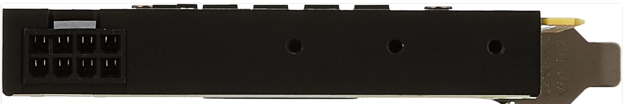
Image 4.5: Side view of the PNY NVIDIA Quadro RTX 4000 graphics card, illustrating the 8-pin power connector required for operation.
