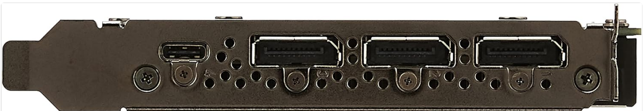
Image 4.4: Rear output panel of the PNY NVIDIA Quadro RTX 4000 graphics card, showing three DisplayPort 1.4 connectors and one VirtualLink (USB-C) port.
