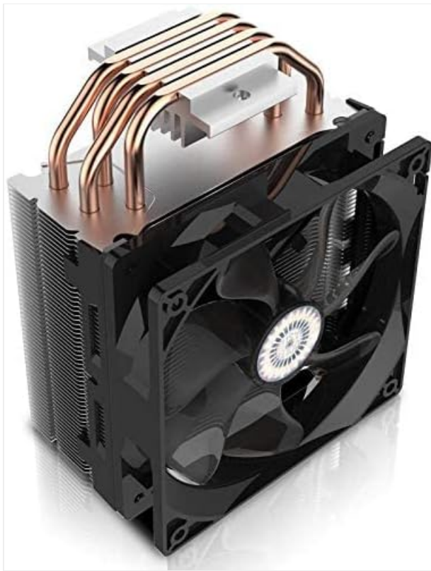
Image: Top-down view of the heatsink, showing the aluminum fins and the ends of the copper heat pipes.
