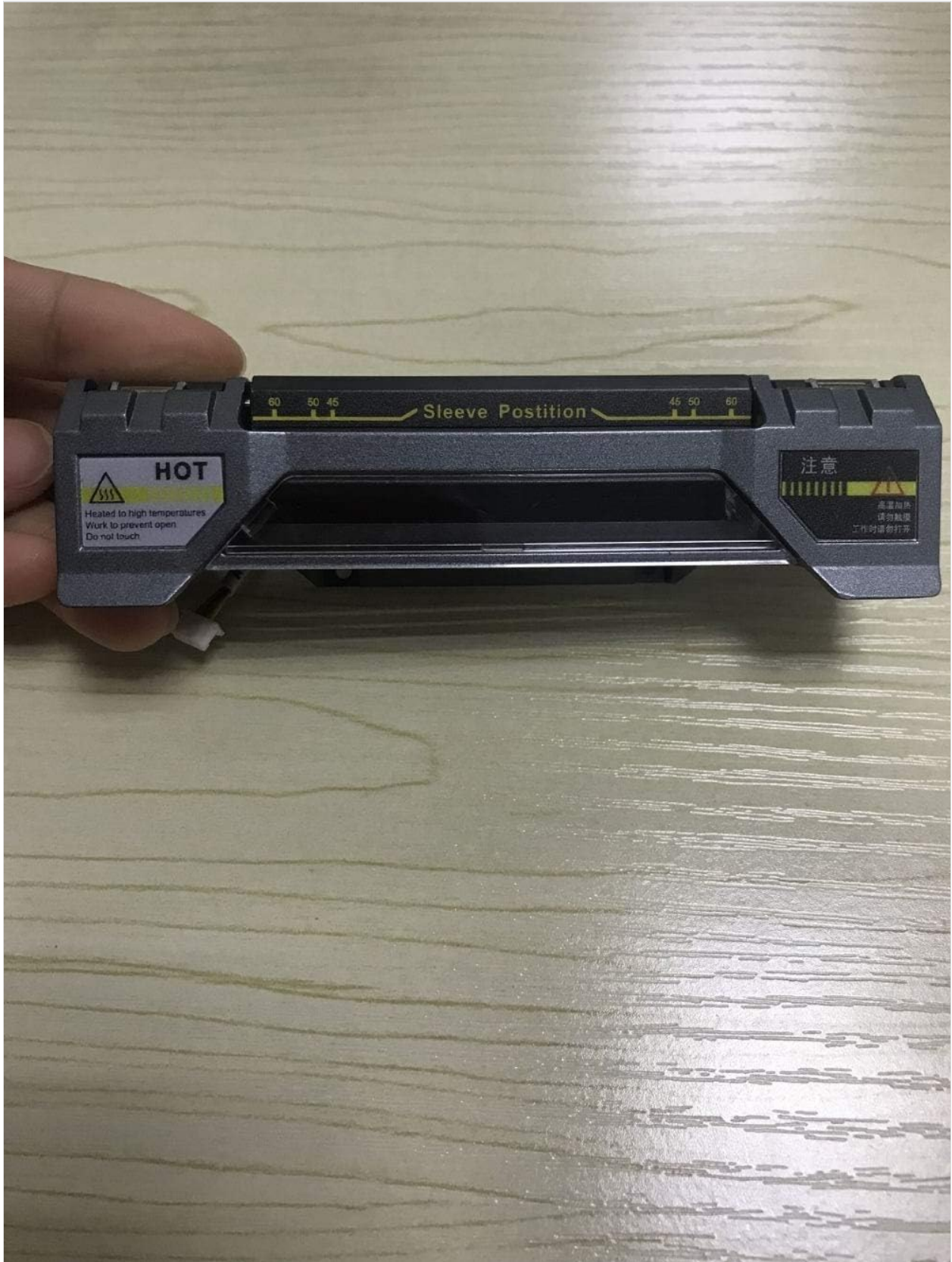
Figure 3.1: Top view of the KOMSHINE FX37 Fiber Optic Heater. This image displays the top surface of the fiber optic heater, highlighting the designated sleeve position area with measurement markings. A clear 'HOT' warning label is visible on the left, indicating high temperatures during operation.
