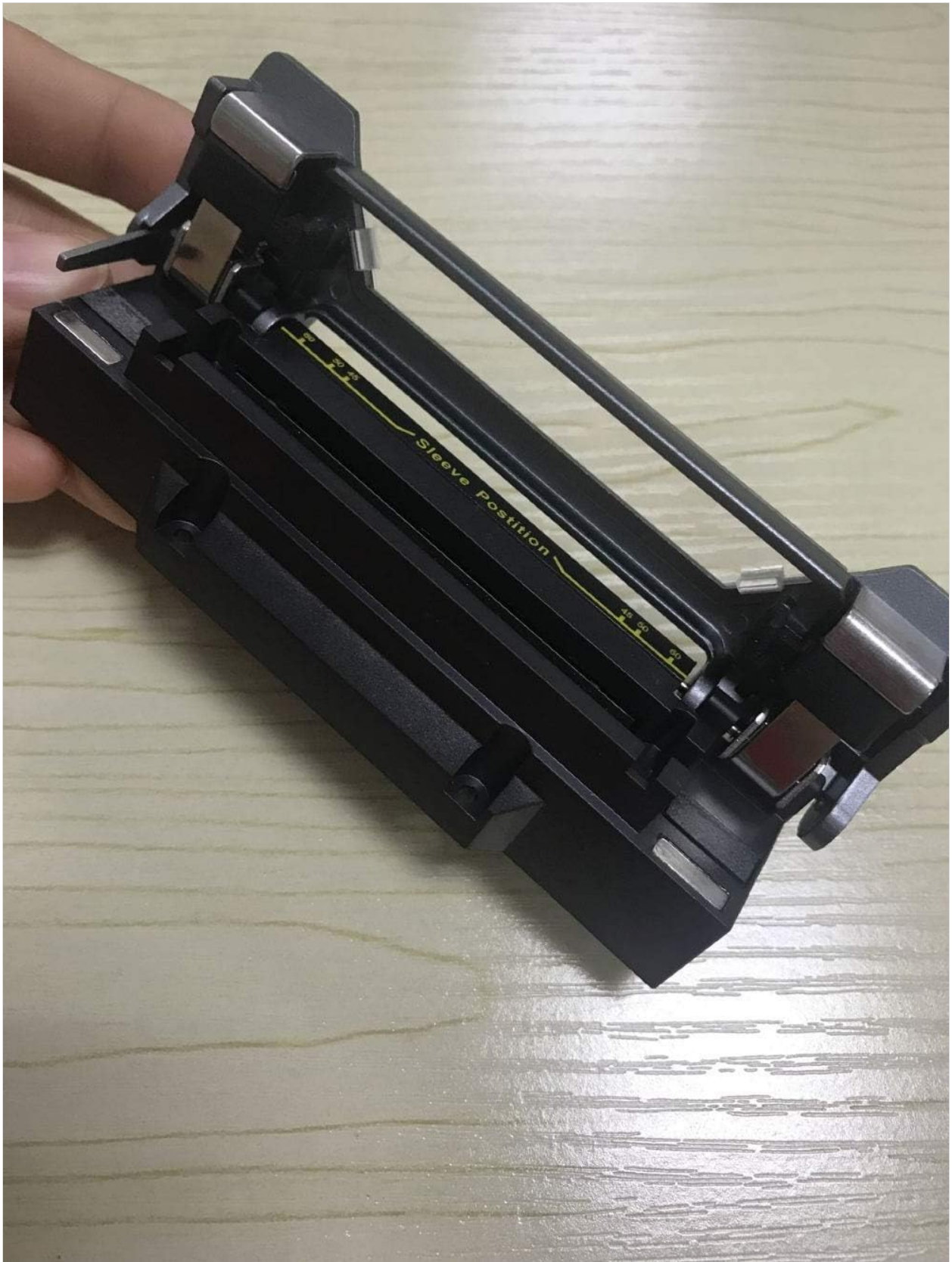
Figure 3.2: Open view of the KOMSHINE FX37 Fiber Optic Heater. This image shows the fiber optic heater with its cover open, exposing the heating chamber where the fiber protection sleeve is placed. The sleeve position guide is clearly visible within the chamber.
