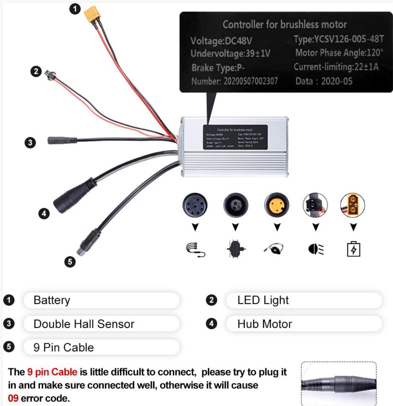
Figure 5.1: BAFANG motor controller with labeled connection points for battery, LED light, Double Hall Sensor, Hub Motor, and 9 Pin Cable.
