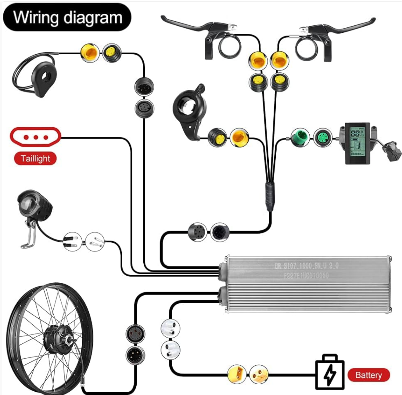
Figure 5.2: Comprehensive wiring diagram illustrating connections between the motor, controller, battery, display, throttle, PAS sensor, headlight, and brake levers.
