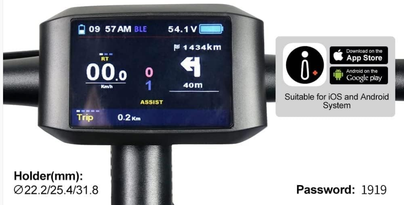
Figure 5.3: BAFANG B750C color display showing various functions like KM/Mile selection, single mileage, total mileage, brightness, auto-off, and brake tips. Also indicates compatibility with iOS and Android systems.
