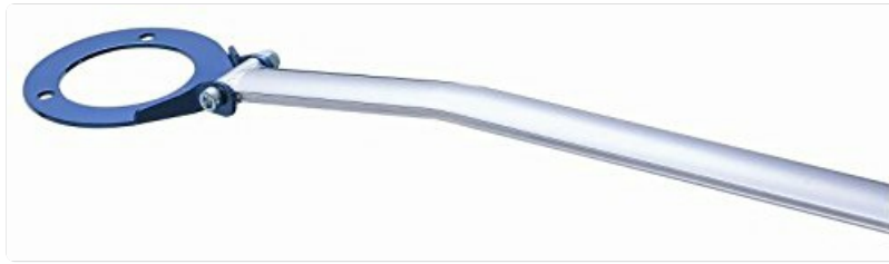
Image 1: Cusco Front Strut Bar OS Type components. This image displays the main oval shaft bar and the blue end brackets, along with associated mounting hardware.
