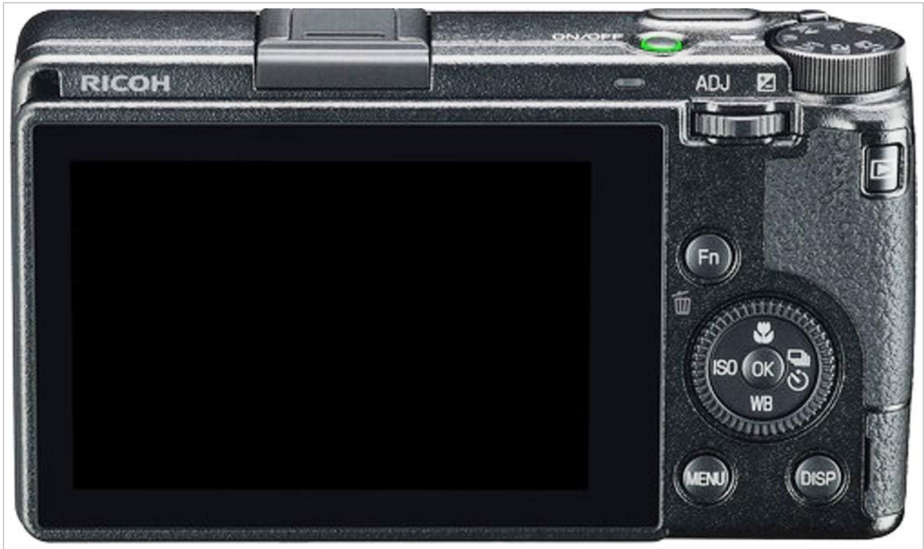
Figure 3.1: Back view of the RICOH GR III, showing the LCD touchscreen and control buttons.
