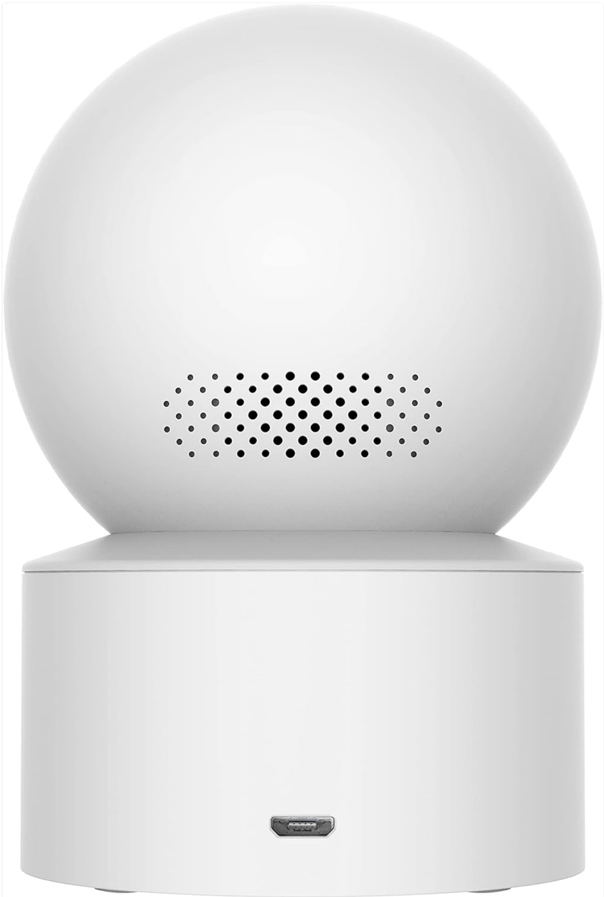
Figure 2: Back view of the Xiaomi Mi Home Cam MJSXJ05CM, highlighting the speaker grille and micro-USB power port.
