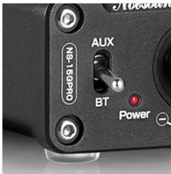
Image 4.1: Close-up of the AUX/BT input selection switch on the amplifier's front panel.
