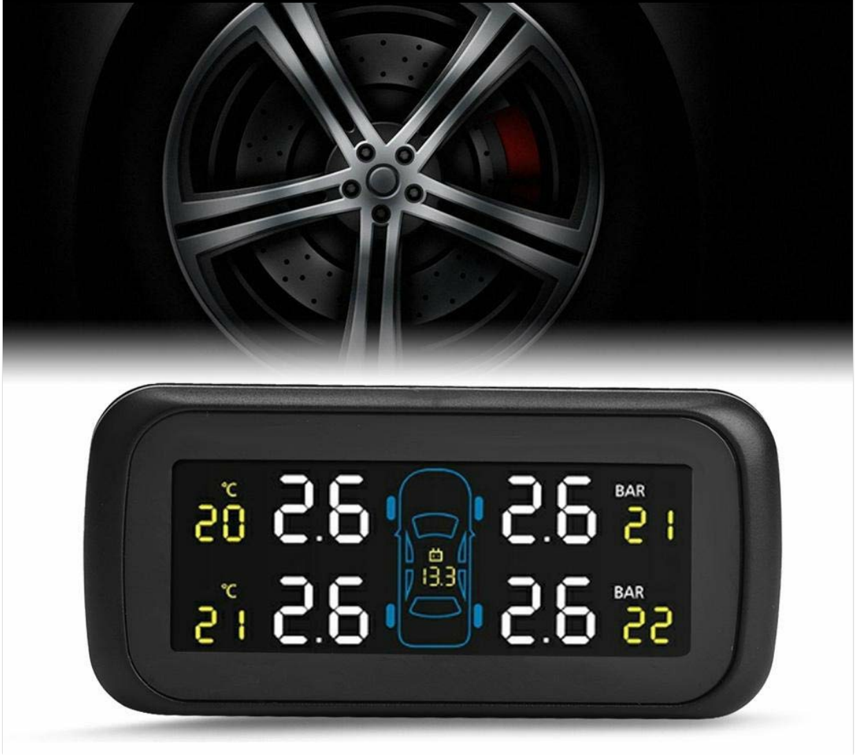
Image 1.1: The Aramox Car TPMS display unit showing real-time tire pressure and temperature for four tires.
