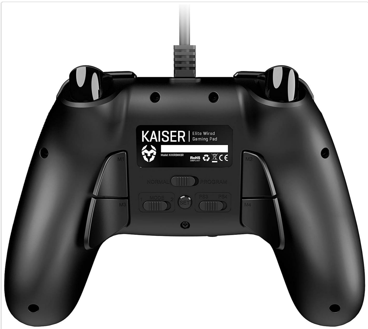
Figure 2: Back View of KROM KAISER Gamepad. This image shows the rear of the gamepad, featuring the four configurable back levers (M1, M2, M3, M4), a Mode switch (Normal/Program), a Set button for configuration, and a switch to select between PS3 and PS4 compatibility modes.
