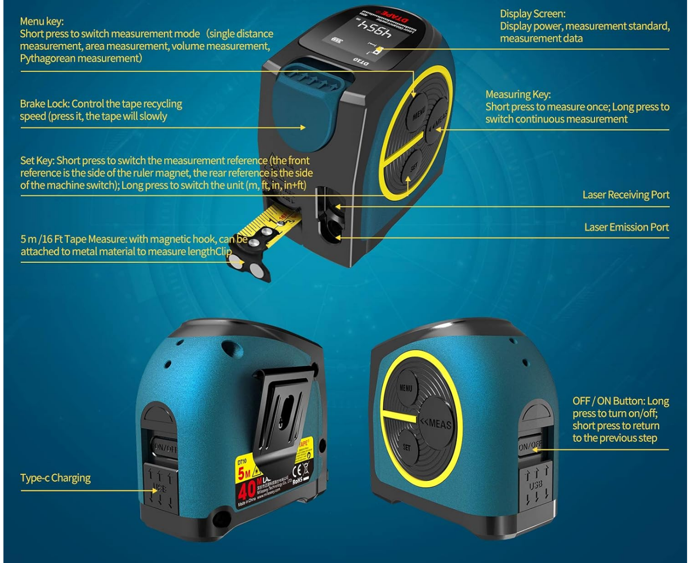
Figure 2: Labeled components of the DTAPE DT10/40M.
