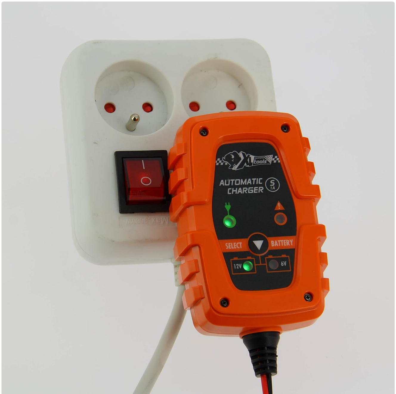
Figure 6.1: The charger indicating operation with a green light when plugged in and connected correctly.
