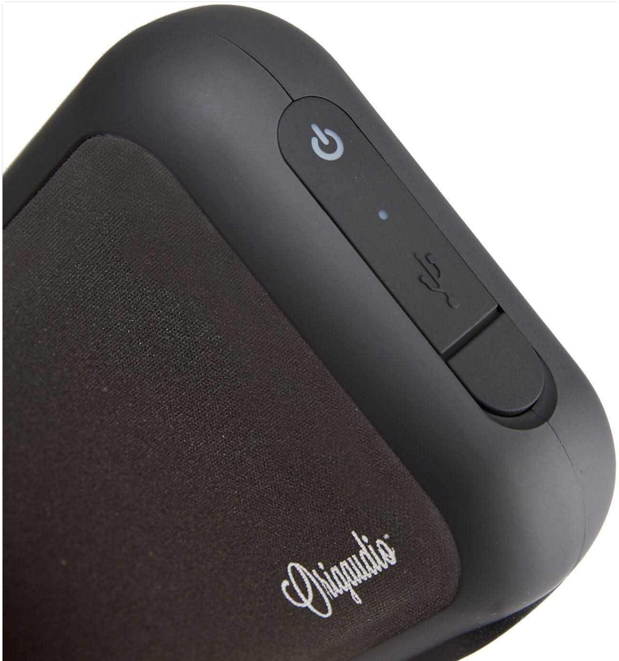
Image: Close-up of the speaker's power button, LED indicator, and Micro USB charging port.
