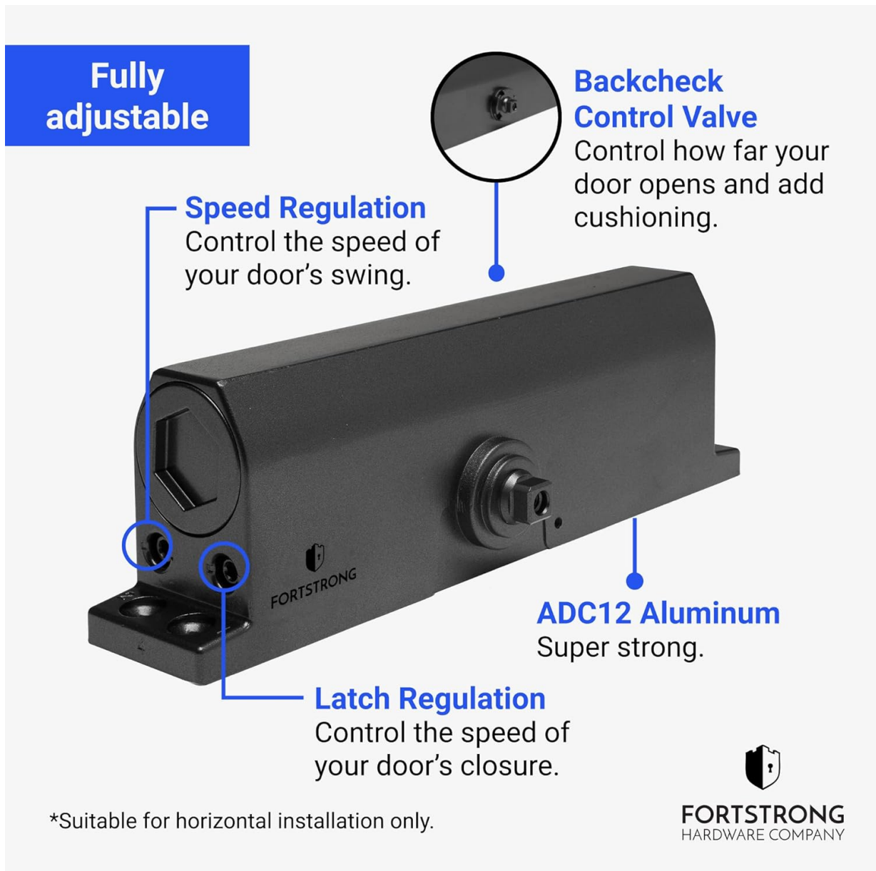
Figure 4.1: Adjustment points on the FS-6300 Door Closer.
