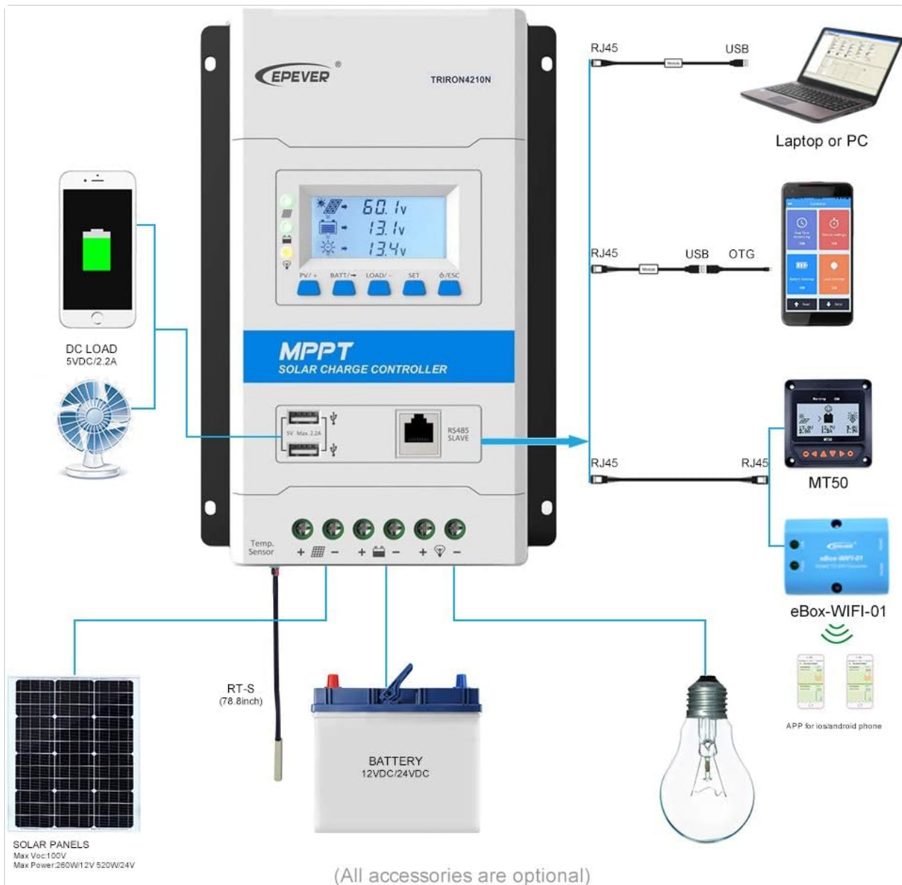
Image: Detailed wiring diagram showing connections for solar panels, battery, and DC load to the TRIRON 4210N controller.
