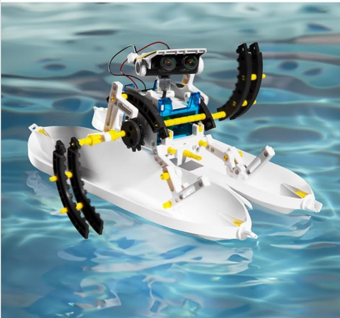
Image: Various SolarBot.14 models demonstrating operation on both land and water surfaces.
