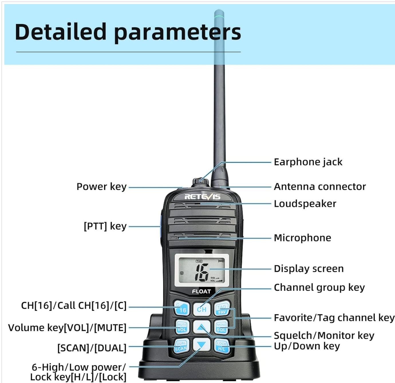
Figure 6: Detailed parameters and button layout of the Retevis RT55 marine radio.
