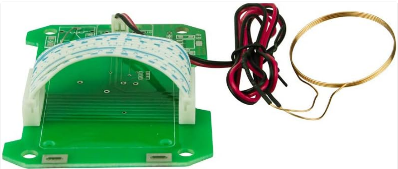
Figure 4: The bypass module's circuit board with the induction coil connected, illustrating the complete internal assembly where the key/chip will be placed.
