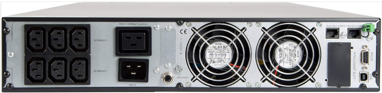
Figure 2.3: Rear panel of the UPS, illustrating the six IEC320 C13-10A output sockets, main power input, cooling fans, USB, RS232, and intelligent slot communication ports.
