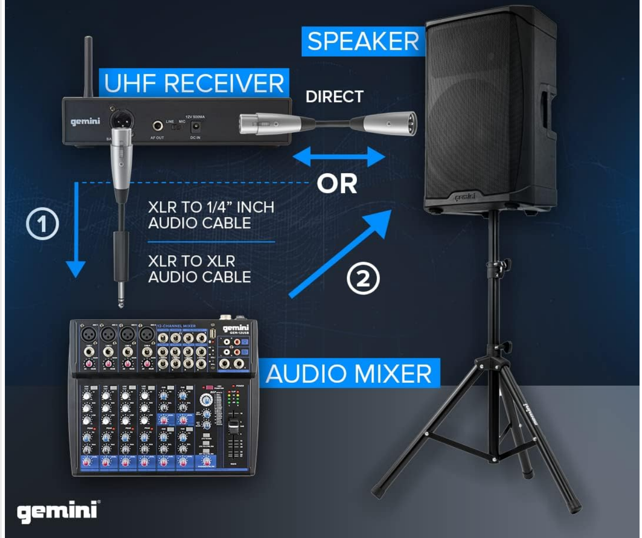
Image 5.1: Connection diagram for the UHF receiver to an audio mixer via XLR or to a powered speaker via 1/4" output.
