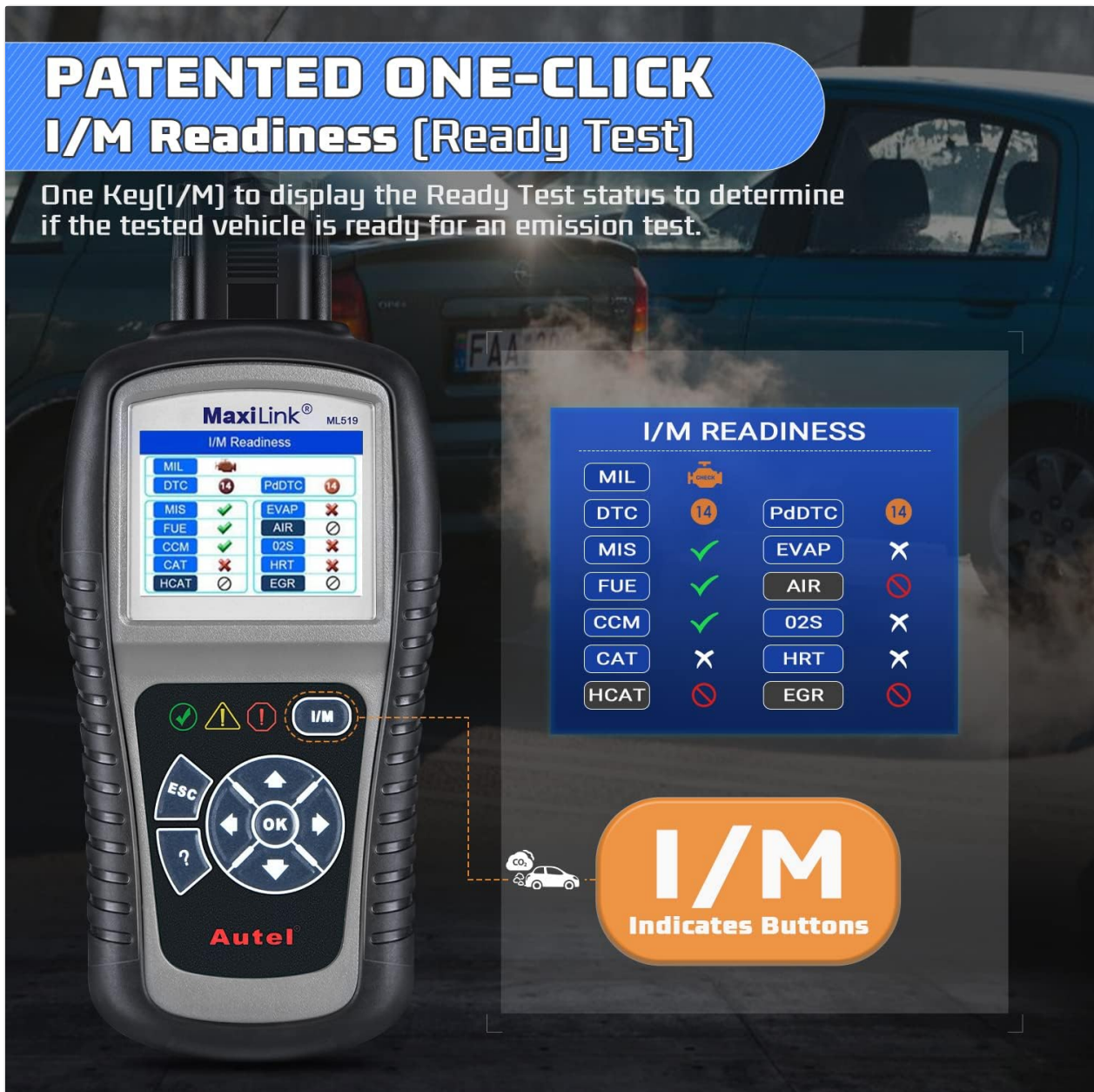
Image: The Autel MaxiLink ML519 displaying the I/M Readiness screen, showing the status of various emission monitors with checkmarks and 'X' symbols.
