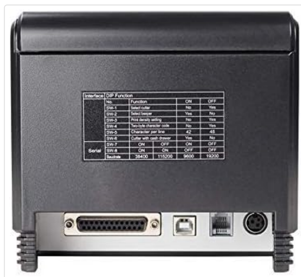
Figure 4: Rear view of the Xprinter Q200, displaying the various connectivity ports and the DIP switch configuration table.
