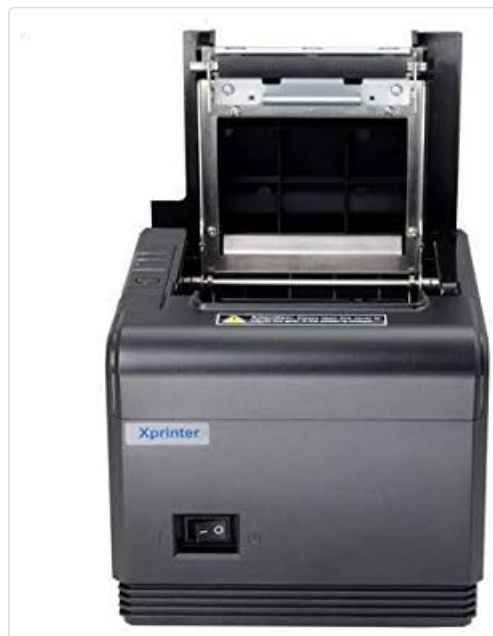
Figure 3: Top view of the Xprinter Q200 with the paper cover open, revealing the thermal paper compartment and the print head mechanism.
