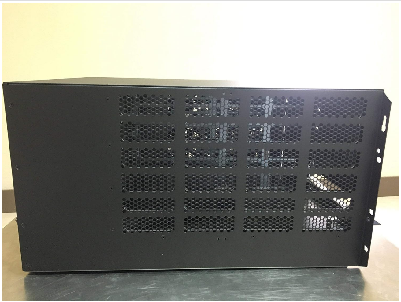
Figure 8.2: Side view of the Brocade FastIron SX 800 chassis, showing extensive ventilation grilles along the side panel, crucial for heat dissipation.
