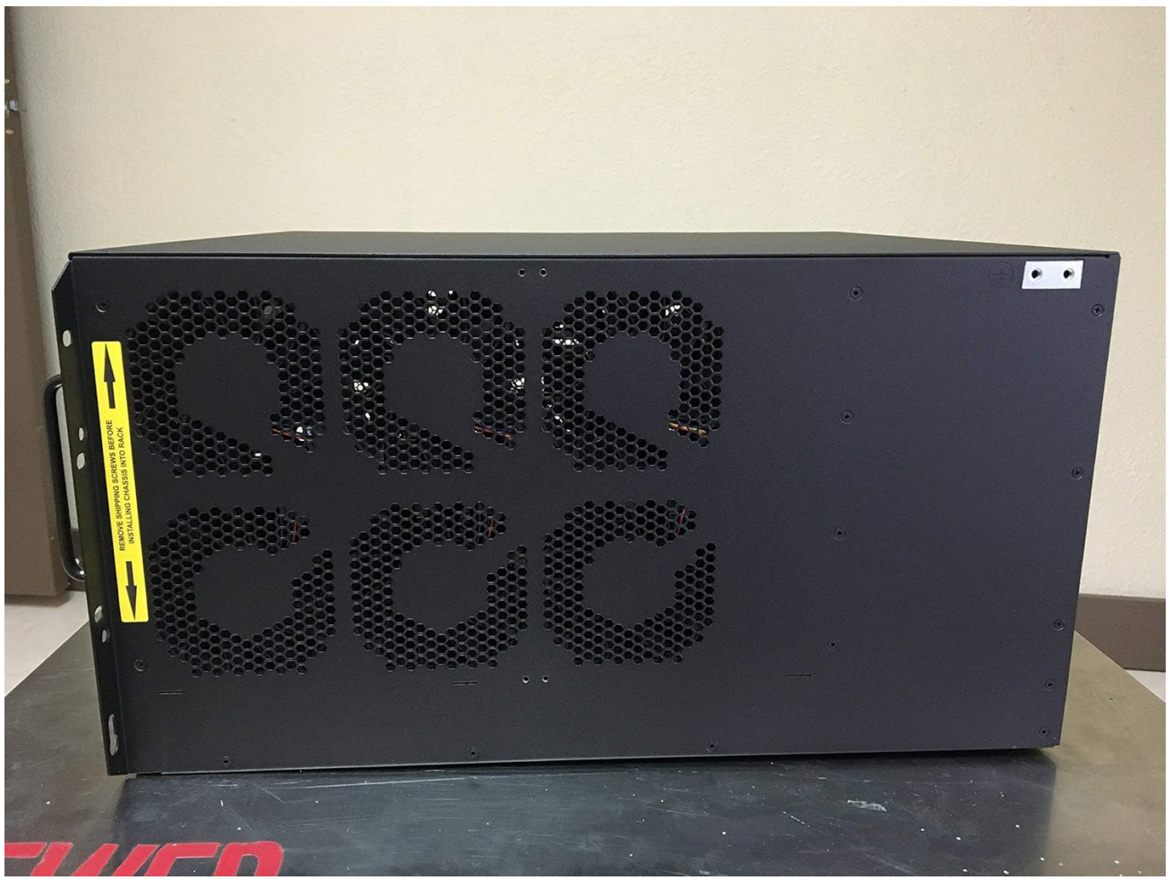
Figure 6.1: Side view of the Brocade FastIron SX 800 chassis, highlighting the fan exhaust grilles and a yellow warning label regarding shipping sleeves. This view emphasizes the cooling system's design.
