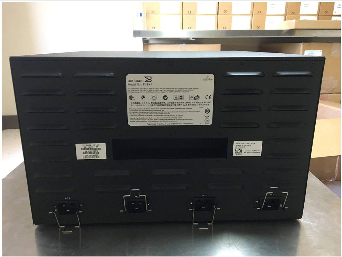
Figure 8.1: Rear view of the Brocade FastIron SX 800 chassis, displaying the multiple AC power input ports and a product label with model and electrical specifications.
