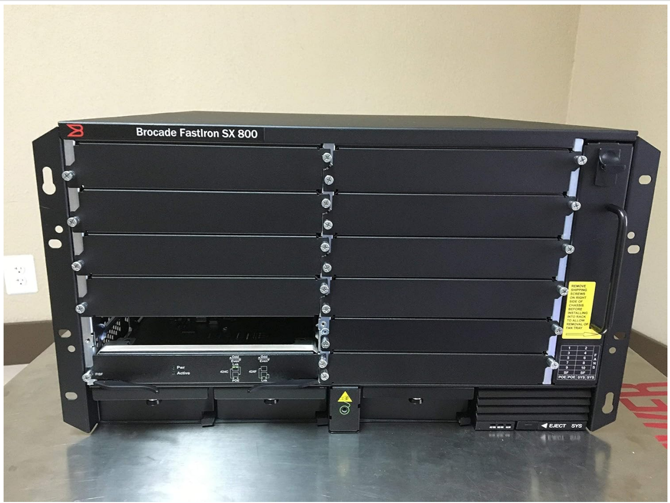
Figure 2.1: Front view of the Brocade FastIron SX 800 chassis, showing the modular slots and power/active indicators. This image displays the main unit with multiple empty slots for modules and a power supply unit installed at the bottom.
