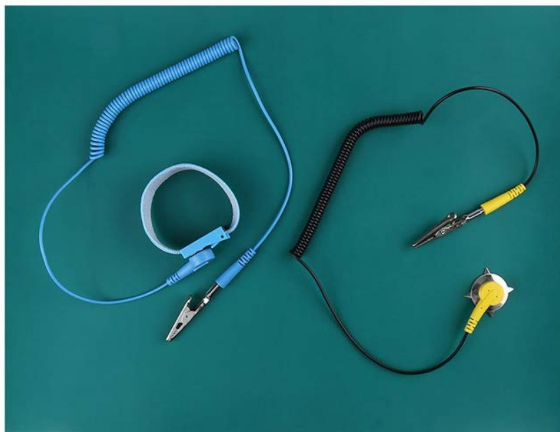
Figure 3.2: Detailed view of the wrist strap, ground clip, and grounding plug.
