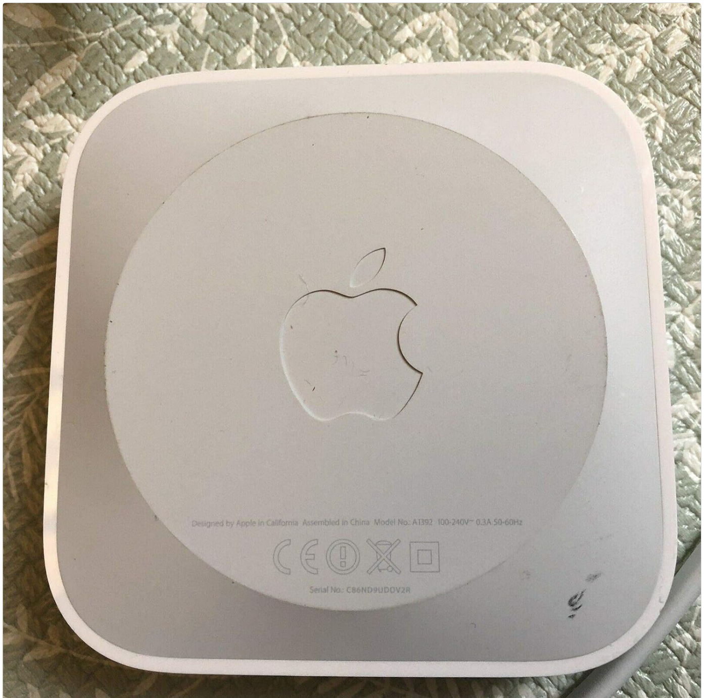
Figure 3.2: The bottom of the AirPort Express A1392, displaying regulatory information, the model number (A1392), and the serial number. The Apple logo is prominently featured in the center.
